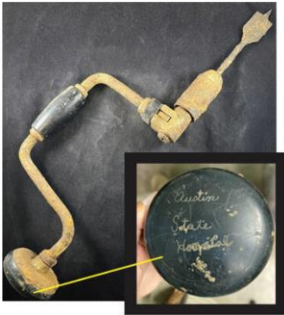
Above: Carpenters would use a metal and plastic brace and bit to drill holes. Power tools were not widely available until the early- to mid-20th century.
